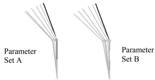
Fig. 4. Final states (grey) after training for 1, 10, 50, 100, and 200 episodes (left to right), where the black state is the goal. The plot on the left uses learning parameter set A, and the plot on the right uses learning parameter set B.
