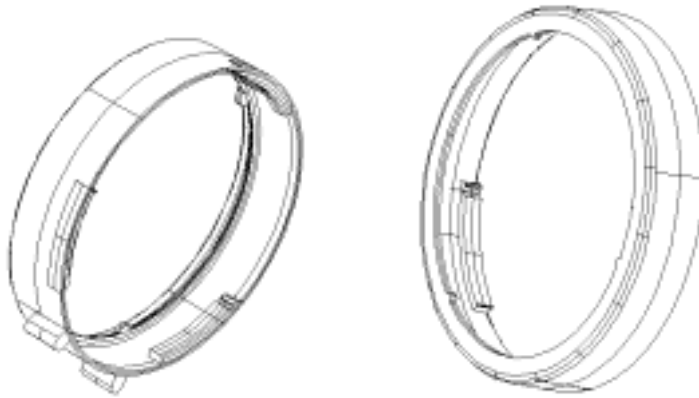
Figure 4-6: CAD Views of the First and Second Generation Concept Reflectors
