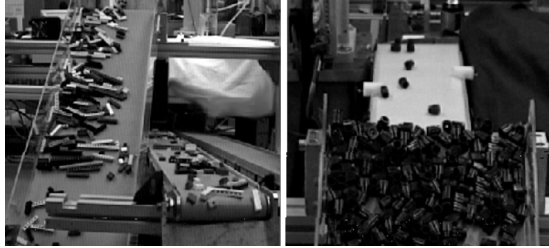
Figure 3: left: LEGO blocks drawn from the hopper and ascending the inclined conveyor right: Sockets spilling from the inclined conveyor onto the horizontal conveyor
